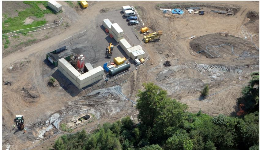
The site compound establishment included a container surrounded pfa storage area and grout mixing area. The containers, set 2 high, provided PFA bunkering but also worksite screening and noise and dust attenuation to the adjacent residential property. Cement was stored in a 30tonne silo.
